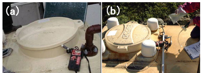
Fig.1 Photographs showing measurement and sampling of methane in the water tank on-site
