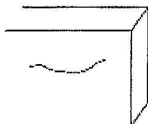
—急速な打込み—
