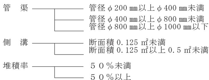
$$(\text{管渠清掃}) \text{ 堆積率 } (\%) = \text{堆積土厚} / \text{管径} \times 100$$
