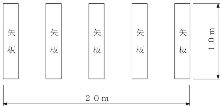
$$\text{基礎用鋼材敷設面積} = 10 \times 20 = 200 \text{ m}^2$$
